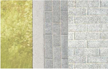
Shared surface Tertiary street materiality option with concrete blocks and flush kerb (not to scale)
