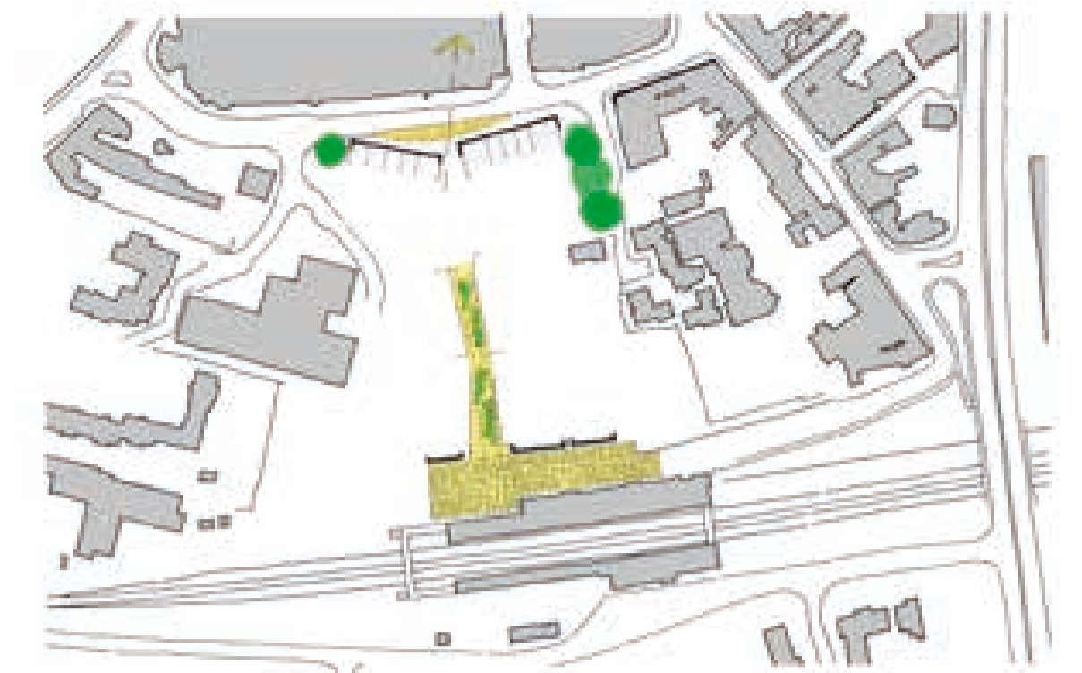
4. Station Walk New pedestrian and cycle north-south street. Enclosure of 1.2:1 is narrower than Bartholomew Street and Cheap Street as it is less important.
