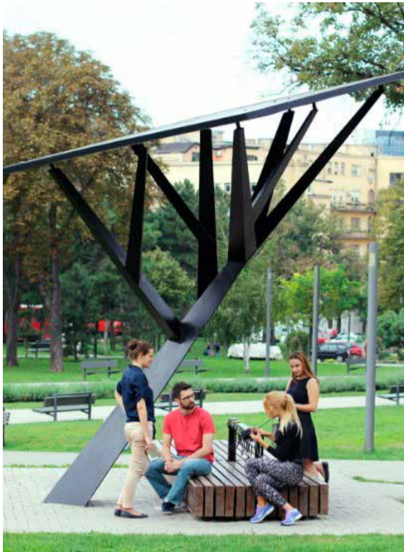
Smart Furniture: Multi functional furniture providing wi-fi hotspots, solar powered charging points for electrical devices. These devices typically contain air quality sensors to monitor environmental changes
